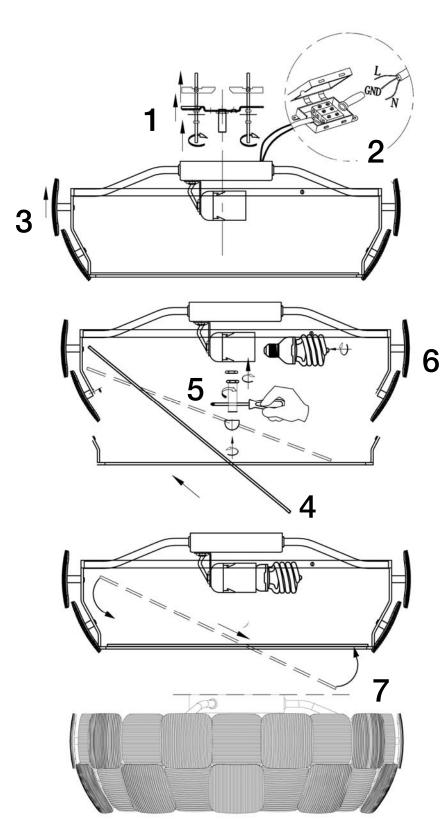
NOTE: For safety reasons, if the electrical wire of this item has any damage, it must be repaired by qualified staff.
